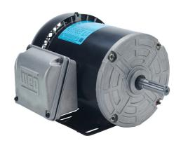
WEG Electric S standard efficiency AC induction motor, general purpose and inverter rated, 1/2hp, 3-phase, 208-230/460 VAC, 3600rpm, TEFC, 56 frame, rolled steel, rigid base mount.
