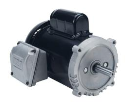
WEG Electric S standard efficiency AC induction motor, general purpose, 1/2hp, 1-phase, 115/208-230 VAC, 3600rpm, TEFC, NEMA 56C frame, rolled steel, C-face mount.
