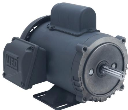
WEG Electric S standard efficiency AC induction motor, general purpose, 1/2hp, 1-phase, 115/208-230 VAC, 3600rpm, TEFC, NEMA 56C frame, rolled steel, C-face/rigid base mount.
