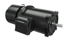
WEG Electric S standard efficiency AC induction motor, general purpose, inverter rated and brake, 1/2hp, 3-phase, 208-230/460 VAC, 1800rpm, TEFC, NEMA 56C frame, rolled steel, C-face mount. Stearns 104817100KQ brake assembly included.
