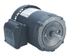
WEG Electric S standard efficiency AC induction motor, general purpose and inverter rated, 1/2hp, 3-phase, 208-230/460 VAC, 1800rpm, TEFC, NEMA 56C frame, rolled steel, C-face mount.
