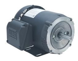
WEG Electric S standard efficiency AC induction motor, general purpose and inverter rated, 1/2hp, 3-phase, 208-230/460 VAC, 1800rpm, TEFC, NEMA 56C frame, rolled steel, C-face/rigid base mount.
