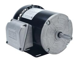
WEG Electric S standard efficiency AC induction motor, general purpose and inverter rated, 1/2hp, 3-phase, 208-230/460 VAC, 1800rpm, TEFC, 56 frame, rolled steel, rigid base mount.
