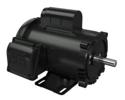
WEG Electric S standard efficiency AC induction motor, general purpose, 1/2hp, 1-phase, 115/208-230 VAC, 1800rpm, TEFC, NEMA 56C frame, rolled steel, C-face/rigid base mount.
