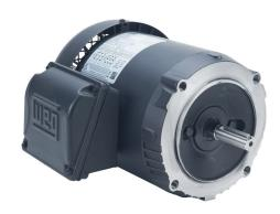
WEG Electric S standard efficiency AC induction motor, general purpose and inverter rated, 1/3hp, 3-phase, 208-230/460 VAC, 3600rpm, TEFC, NEMA 56C frame, rolled steel, C-face mount.
