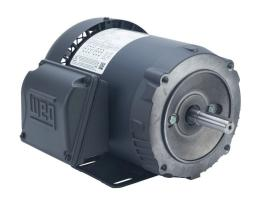
WEG Electric S standard efficiency AC induction motor, general purpose and inverter rated, 1/3hp, 3-phase, 208-230/460 VAC, 3600rpm, TEFC, NEMA 56C frame, rolled steel, C-face/rigid base mount.
