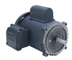
WEG Electric S standard efficiency AC induction motor, general purpose, 1/3hp, 1-phase, 115/208-230 VAC, 3600rpm, TEFC, 56C frame, rolled steel, C-face mount.
