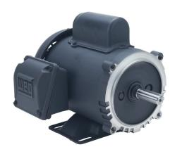
WEG Electric S standard efficiency AC induction motor, general purpose, 1/3hp, 1-phase, 115/208-230 VAC, 3600rpm, TEFC, NEMA 56C frame, rolled steel, C-face/rigid base mount.
