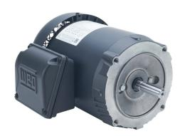
WEG Electric S standard efficiency AC induction motor, general purpose and inverter rated, 1/3hp, 3-phase, 208-230/460 VAC, 1800rpm, TEFC, 56C frame, rolled steel, C-face mount.
