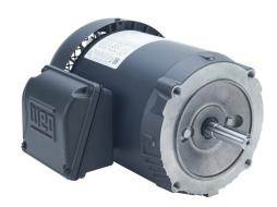
WEG Electric S standard efficiency AC induction motor, general purpose and inverter rated, 1/3hp, 3-phase, 208-230/460 VAC, 1800rpm, TEFC, NEMA 56C frame, rolled steel, C-face mount.
