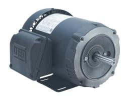
WEG Electric S standard efficiency AC induction motor, general purpose and inverter rated, 1/3hp, 3-phase, 208-230/460 VAC, 1800rpm, TEFC, NEMA 56C frame, rolled steel, C-face/rigid base mount.
