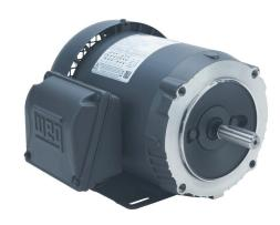
WEG Electric S standard efficiency AC induction motor, general purpose and inverter rated, 1/4hp, 3-phase, 208-230/460 VAC, 3600rpm, TEFC, 56C frame, rolled steel, C-face/rigid base mount.
