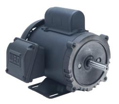
WEG Electric S standard efficiency AC induction motor, general purpose, 1/4hp, 1-phase, 115/208-230 VAC, 3600rpm, TEFC, NEMA 56C frame, rolled steel, C-face/rigid base mount.
