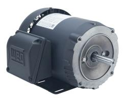
WEG Electric S standard efficiency AC induction motor, general purpose and inverter rated, 1/4hp, 3-phase, 208-230/460 VAC, 1800rpm, TEFC, NEMA 56C frame, rolled steel, C-face/rigid base mount.
