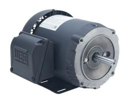
WEG Electric S standard efficiency AC induction motor, general purpose and inverter rated, 1/4hp, 3-phase, 208-230/460 VAC, 1800rpm, TEFC, 56C frame, rolled steel, C-face/rigid base mount.
