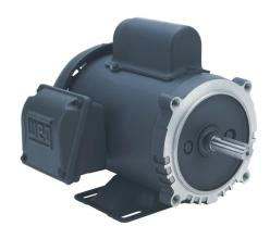
WEG Electric S standard efficiency AC induction motor, general purpose, 1/4hp, 1-phase, 115/208-230 VAC, 1800rpm, TEFC, NEMA 56C frame, rolled steel, C-face/rigid base mount.
