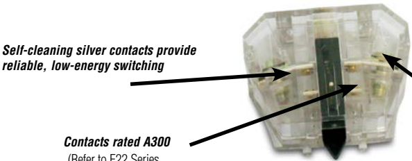
Clear contact block for illustration purposes. Clear contact blocks are not available for sale from AutomationDirect.
