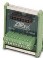
ZL-RTB20 20-pin feed-through connector module
