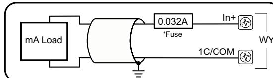
\*An Edison S500-32-R 0.032A fast-acting fuse is recommended for all analog voltage inputs, analog outputs, and current loops.
