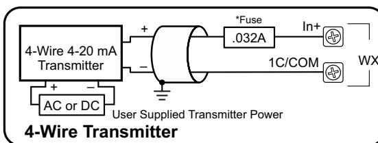
NOTE: Shield should be connected only at one end, to ground at the source device.
