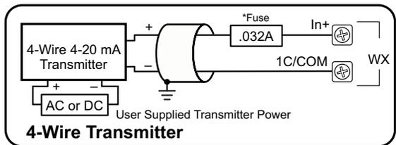
**NOTE:** Shield should be connected only at one end, to ground at the source device.
