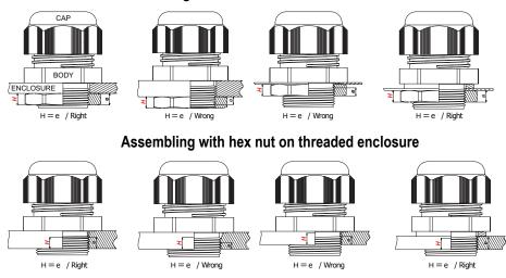
• The engaged thread length "e" must be equal or longer than relevant hex nut thickness "H"
