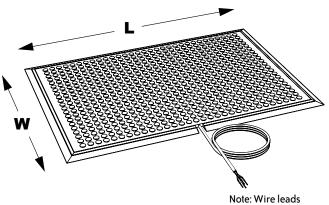
SENTIR safety contact mats are laminar sections which are used to safeguard dangerous areas in industrial and production automation settings. Stepping on the mat triggers an immediate "stop" signal in order to prevent endangering movements.
