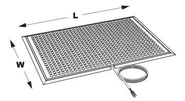
Use wire leads brown and blue (1 & 3) for continuity and white and black (2 & 4) for continuity. (See safety relay for wiring) SENTIR safety contact mats are rectangular sections which are used to safeguard dangerous areas in industrial and production automation settings. Stepping on the mat triggers an immediate "stop" signal in order to prevent endangering movements.
