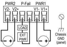
Optional Dual DC Supplies \*Fault Contact opens when in a faulted state
