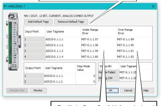
The "Under Range Error" bit for each channel activates for a signal around 0mA ± offset error.
