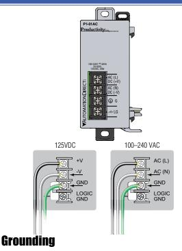
A good common ground reference (earth ground) is essential for proper operation of the Productivity1000 system. One side of all control circuits, power circuits and the ground lead must be properly connected to earth ground by either installing a ground rod in close proximity to the enclosure or by connecting to the incoming power system ground. There must be a single-point ground (i.e. copper bus bar) for all devices in the enclosure that require an earth ground.
