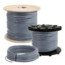
Control and signal cable from Quabbin is available in sizes from 24 AWG to 16 AWG with up to 25 conductors. These are available either in unshielded or shielded constructions. Individual conductors are stranded tinned copper with color coded insulation for easy identification, with an industry standard PVC chrome gray jacket. Shielded versions include an overall aluminum mylar foil tape with a tinned copper drain wire for maximum effectiveness against external electrical noise interference.
