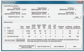
Ethernet I/O Monitor offers unparralled visibility of all traffic on your Ethernet I/O network. Identify specific problems at a glance and jump to the System Configuration or Viewing screens with a single click.
