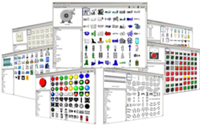
Figure 1: Typical HMI objects. HMI development environments typically provide many design elements representing physical devices, like valves and pumps, and logical devices, like analog meters. Some samples of the AutomationDirect C-more development software are shown here.
