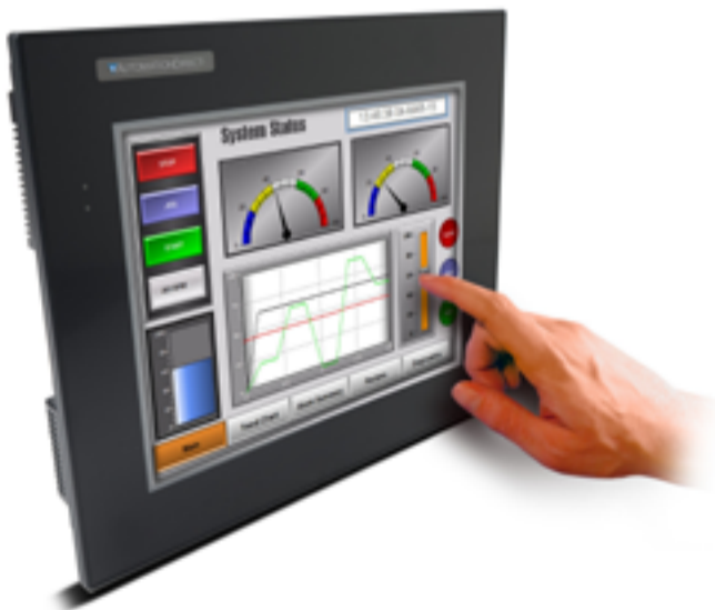
Figure 3: Image of a configured HMI in use. Developing and following an HMI style guide will allow designers to configure intuitive HMI screens which operators can easily navigate to monitor and control factory automation systems.
