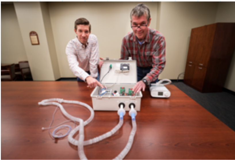
Figure 5: Dr. Michael Zabala (at left) and Dr. Thomas Burch (at right) demonstrate the RE-INVENT, which is built from commercial off-the-shelf parts to adapt a common CPAP machine into a ventilator.
