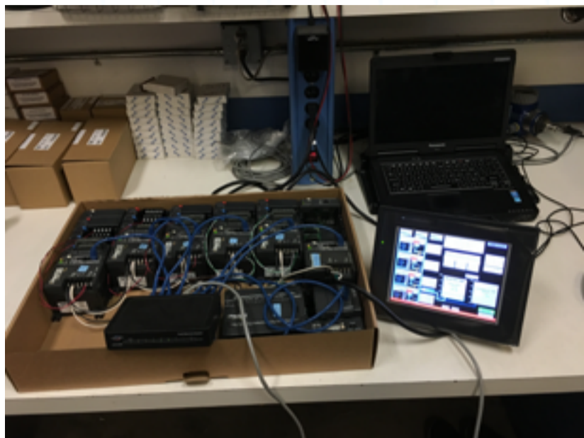
Figure 3: PLC/HMI test bench. Helix performed extensive bench testing to ensure their AutomationDirect PLC programming and HMI configurations would control locally as needed while communicating as required.
