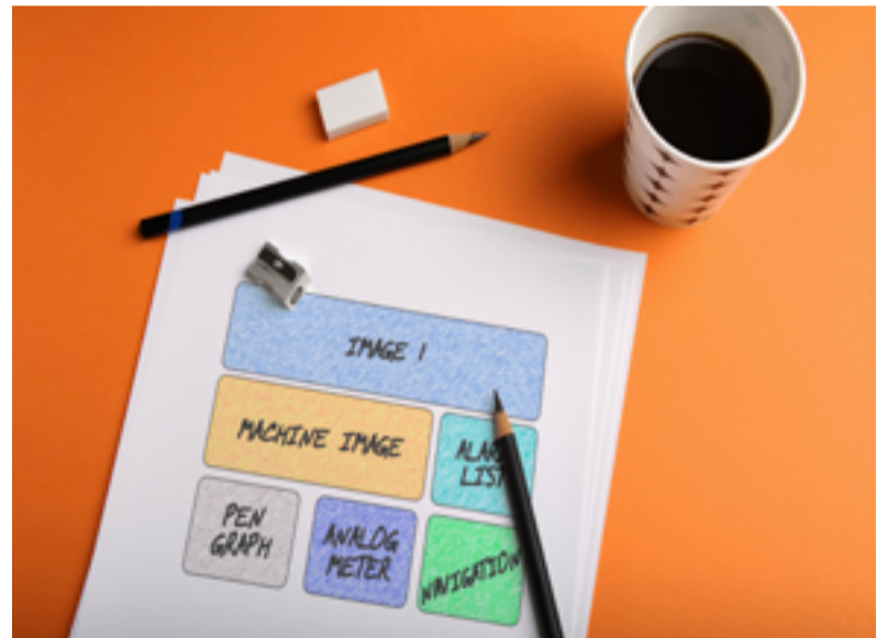
Figure 2: Story board image. Story boards allow HMI designers to pre-plan interface requirements and get approval before expending significant configuration effort.
