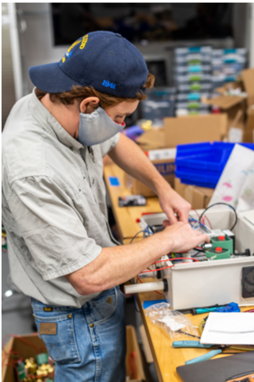
Figure 1: For early-generation CPAP-based ventilator designs, the team prototyped with basic and readily available parts.
