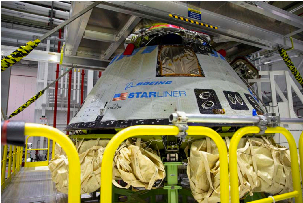
The Boeing CST-100 Starliner spacecraft at the company's Commercial Crew and Cargo Processing Facility in Florida, undergoing inspection after its Orbital Flight Test. (Photo Credit: NASA/Frank Michaux)
