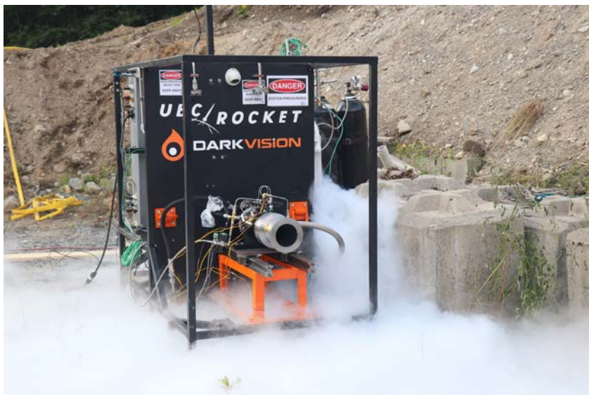
Figure 1: Picture of rocket test stand venting tanks after a hot fire. The rocket engine, shown here attached to the test stand, must be controlled to carefully combine and ignite liquid oxygen and kerosene while monitoring results.
