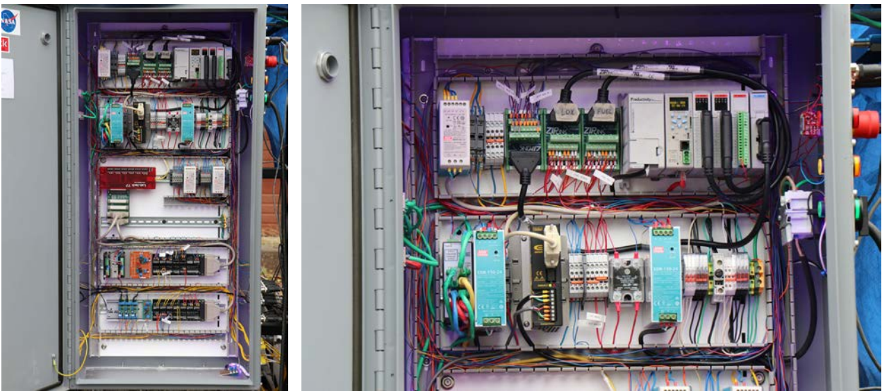
Figure 2: Picture of control panel. The team designed, fabricated, and wired a control panel mounted on-board the test stand, featuring an AutomationDirect Productivity2000 PLC, with ZIPLink connector cables installed at the top.
