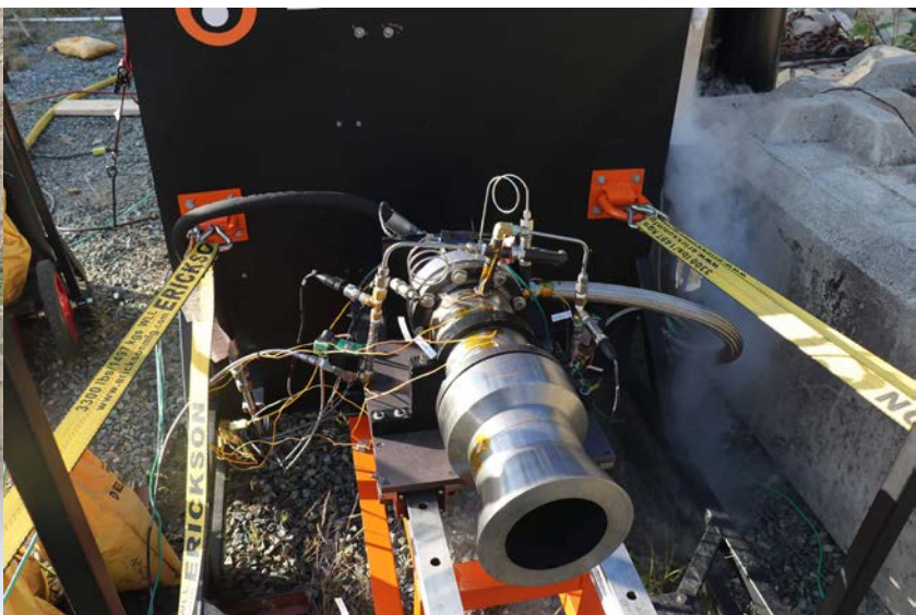
Figure 1: Picture of rocket test stand venting tanks after a hot fire. The rocket engine, shown here attached to the test stand, must be controlled to carefully combine and ignite liquid oxygen and kerosene while monitoring results.
