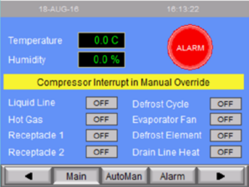
Figure 4: (courtesy of Affinity Energy) The AutomationDirect C-more HMI's main status screen provides temperature and humidity indication, along with field device status.
