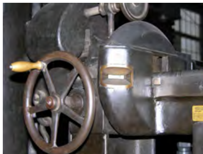
Image 6: The counterweight crank drive and dial indicator displaying in 10lb increments
