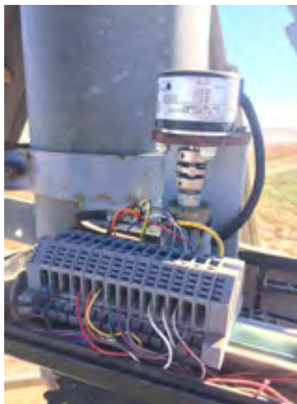
Image 3: The Carter pivot irrigation system makes use of a zero lash coupler to attach the systems sprocket shaft to an absolute encoder.
