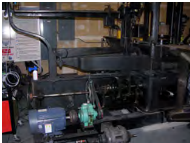
Image 4: The beam testing machine drive train features 4-speed transmission, ring and pinion gear assembly, V-belt pulley drive, 5 hp AC motor with VFD, and a reversible gearbox.
