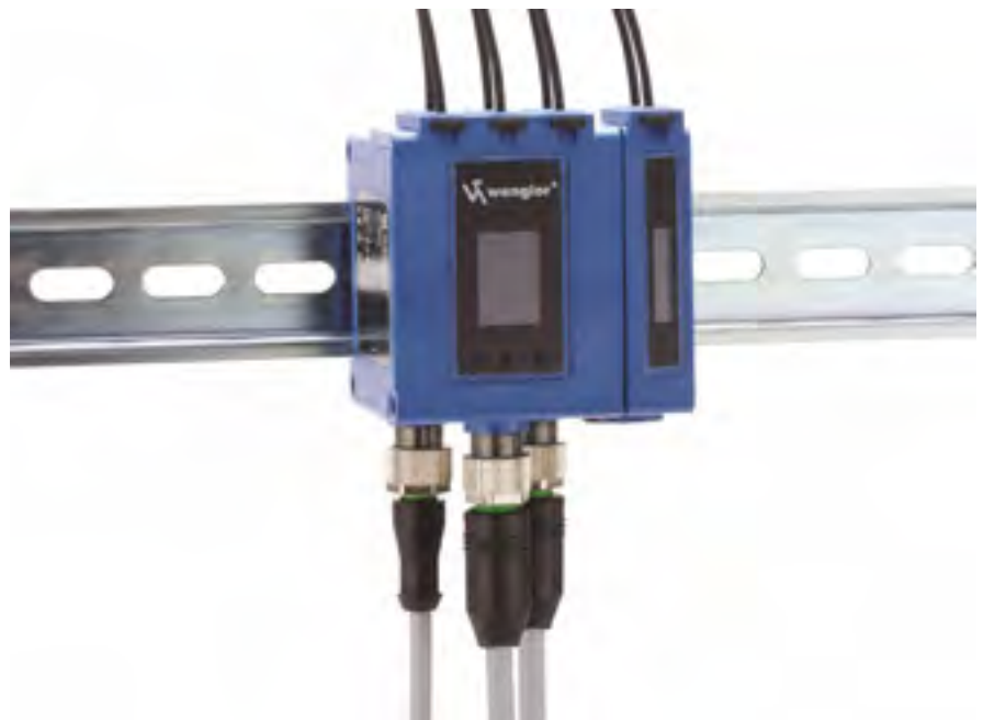
Figure 3: Fiber optic manifolds with expansion electronics simplify and reduce the number of wires to the machine controller by converting sensor signals to digital data, and combining signals logically if desired. Pictured is AutomationDirect's new three-channel OPT2042 fiber manifold which is expandable to 15 channels. It accepts various plastic and glass fiber optics, and transmits and receives data via IO-Link to allow full 15 channel diagnostics on a single 4-pin connector. It can also be wired with two 8-pin M12 connectors to hardwire each channel if needed, for example in applications where the controller doesn't support IO-Link.
