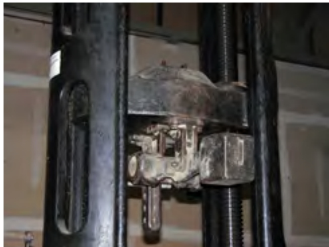
Image 3: The loading assembly consists of the tension frame, lead screw-driven crosshead, loading platform, and side arm supports for long beams.
