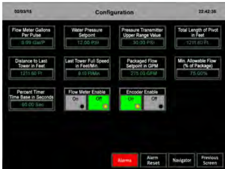
Image 2: The pivot irrigation system can be easily configured, based on the package data provided with the system and selections made by the operator.
