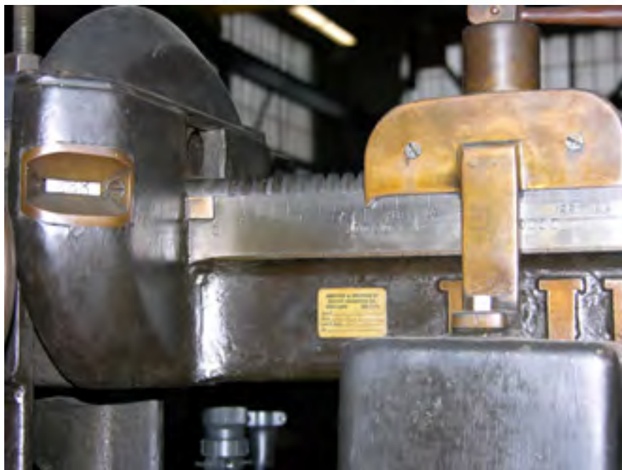
Image 5: The balance system provides the final mechanical advantage that keeps the system in equilibrium.
