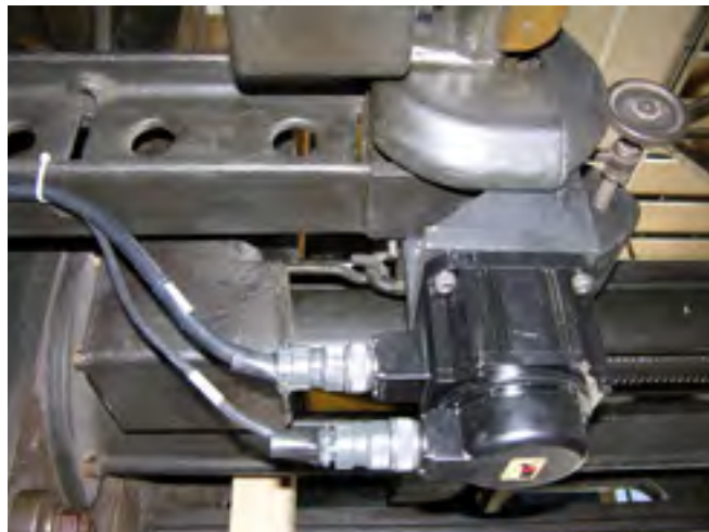
Image 2: A SureServo servo system moves the counterweight to maintain balance.
