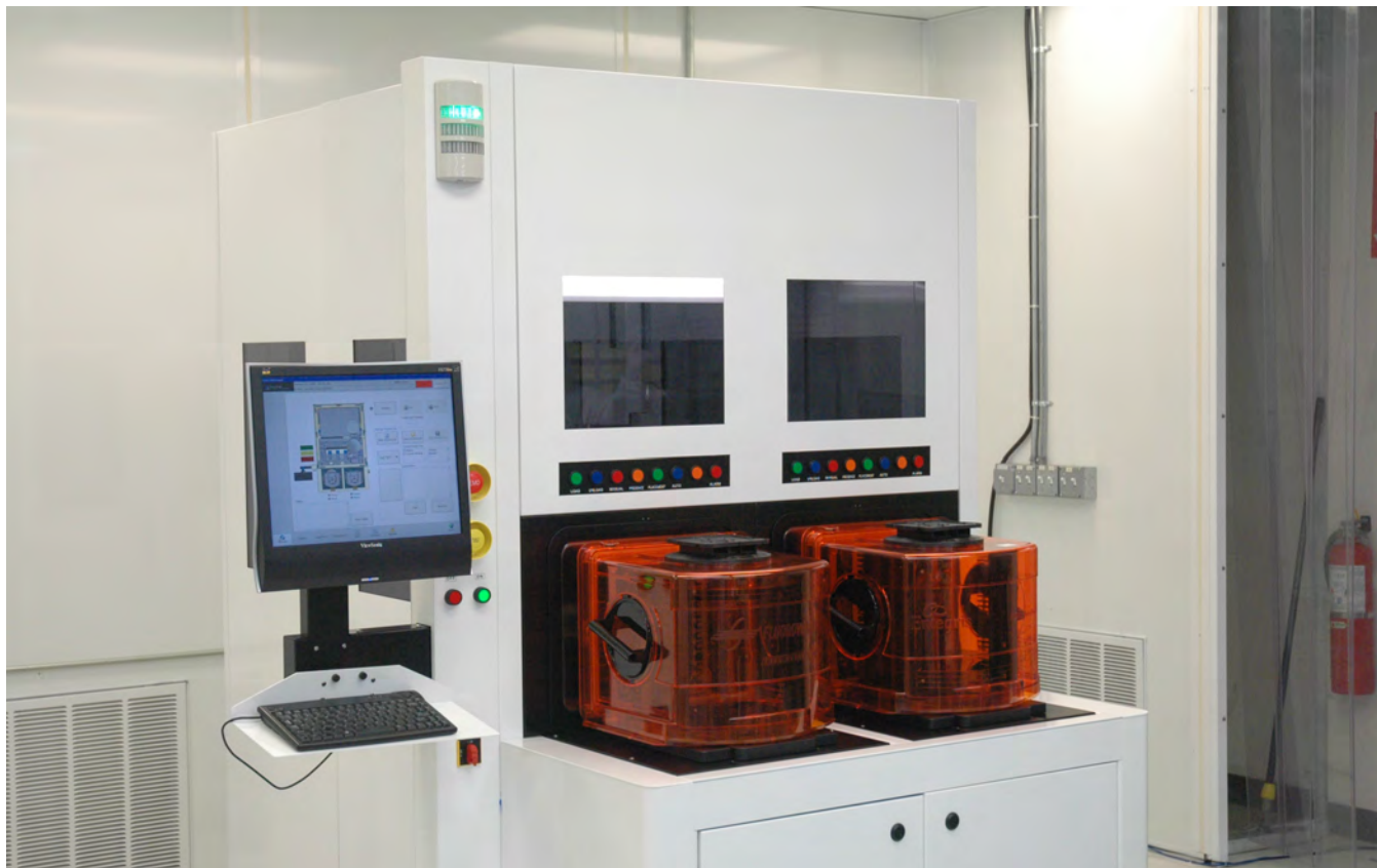
FIGURE 1: This 300mm wafer platform is made by Owens Design and is connected to their customer's IT system via a PC and OPC. (Image courtesy of Owens Design).
