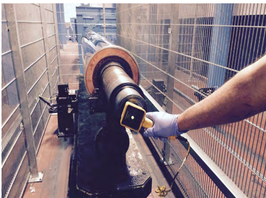
FIGURE 2: Quad Graphics uses a handheld scanner to read data from an RFID tag affixed to print cylinders, allowing inventory tracking. (Image courtesy of TURCK).
