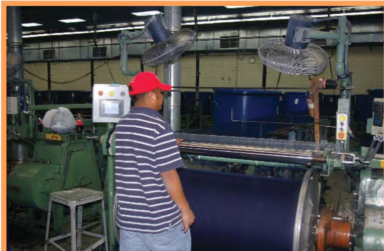
Figures 5 & 6, An operator works the rebeamer during production. The move to a software based C-more has given the operator more capability to change parameters during production.
