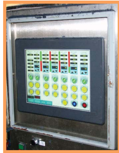
Figure 4, The 15" C-more touch screen operator interface brings all the controls of the finish line to a common point on the machine and includes setup screens, maintenance screens, operations screens as well as diagnostics.
