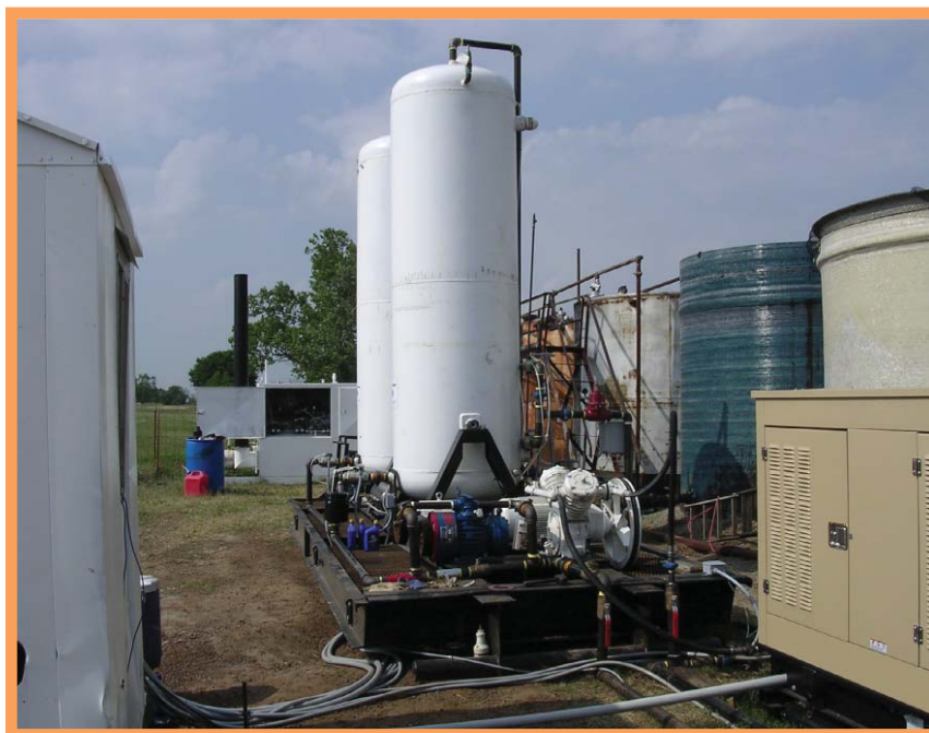
Figure 2, This is a photo of the entire system. The small white house to the left is the control center. The generator on the right runs on gas from the well. The purified natural gas is stored onsite in a huge propane tank. The connection to the gas distribution pipeline is behind the white tanks. This system is designed to run autonomously once started. The only human interaction needed is for someone to check on the generator's engine oil periodically.
