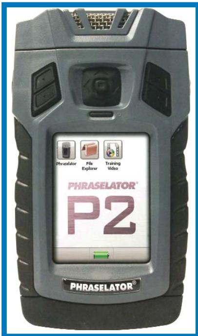
Figure 4, Phraselator automatic verbal translation unit developed by VoxTec, a company begun by a team of ex-Navy SEALs.
