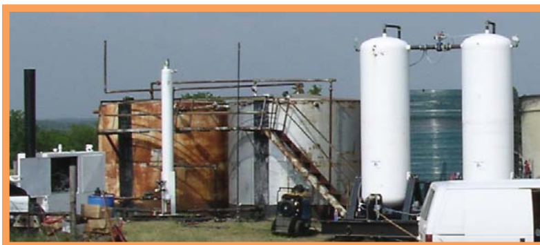
Figure 1, The picture above is of the system on site in Oklahoma. The two large white towers are the adsorbers. The smaller tower is a dehumidifier. The old tanks in the background are the remains of the decommissioned oil facility.
