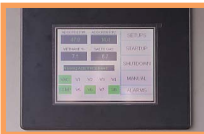
Figure 5, Here is a shot of the screen in action onsite. The interface is as simple as it looks. The idea was that anyone could start the system up, or shut it down with little or no training. All critical values and status are available on this one screen. The STARTUP and SHUTDOWN buttons lead to a series of screens that walk the operator through the proper ways to startup and shutdown the entire system. Status messages appear below the digital displays. The alarm banner is at the bottom of the screen. Once this process has been perfected, many more of these systems can be produced to help meet the energy needs of America.
