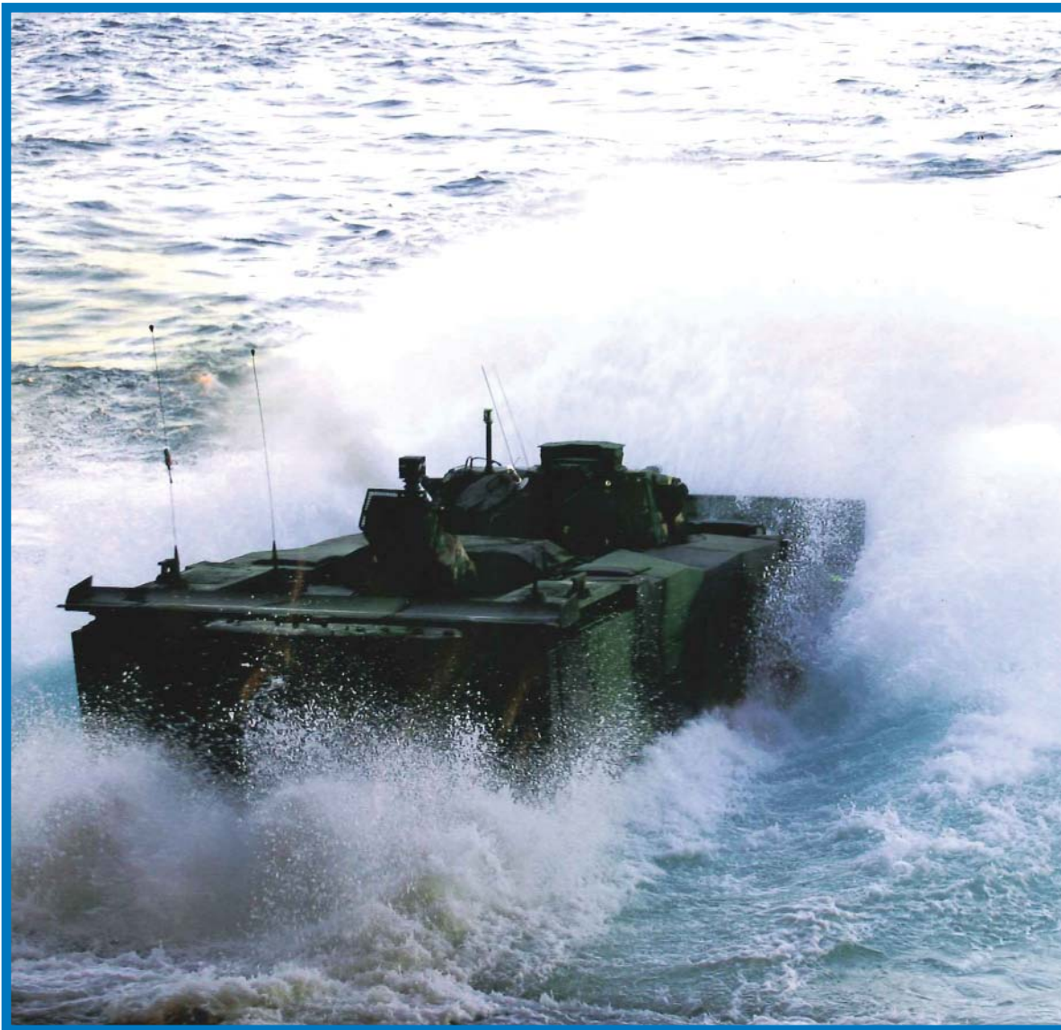
Figure 1, The Marine Corps' new Expeditionary Fighting Vehicle uses waterjets for speeds up to 25 knots in water and up to 45 mph on land.
