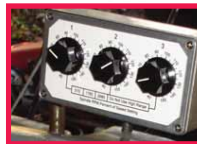
Figure 3, Three potentiometers wired to a shielded cable
