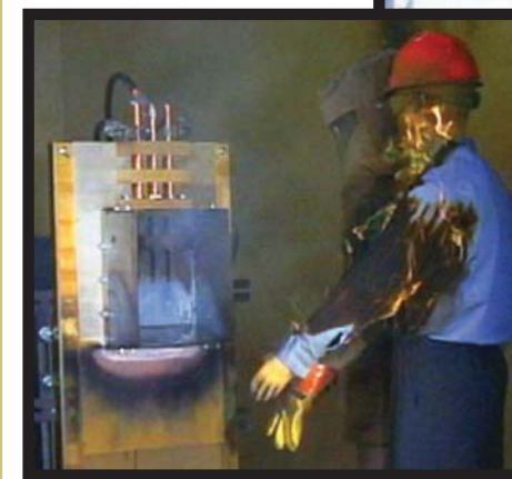
Non-FR work clothing burns after arc exposure
