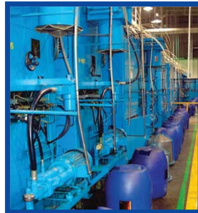
These 7.5 hp motors are driving hydraulic pumps on automated winders in an Emerson Motor Co. plant. Photo courtesy of: Emerson Motor Co., reprint with permission from Plant Engineering
