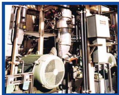
These motors are driving blowers in a chlorine-free pulping process at a paper mill.
