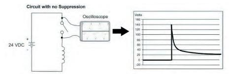
Inductive loads generate transient voltages when their coils are de-energized. These transient voltages can be many times greater than the coil voltage, damaging devices in the circuit and causing unreliable operation in neighboring electronics. It is essential to manage these transients with surge suppressors to extend the life of connected components and provide reliable control system operation.
