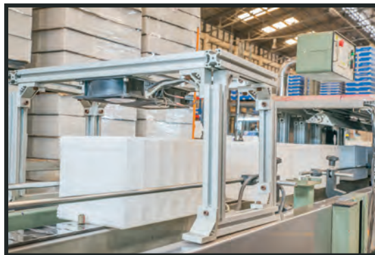
T-Slotted aluminum rail structure holding fans above a conveyor
