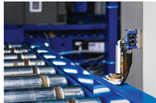
Photoelectric sensors detect object presence or distance in a wide range of industrial applications, and typically contain all required optics and electronics in a single unit.
