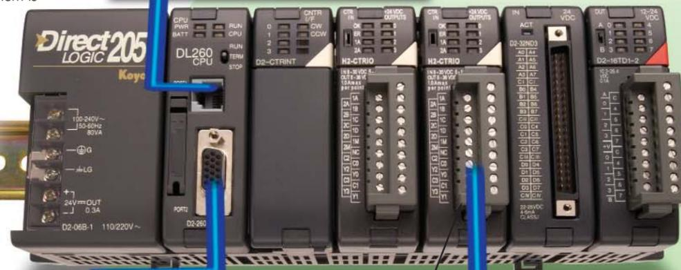
AutomationDirect DL205 PLC with H2-CTRIO module (\$289.00) using pulse output feature
