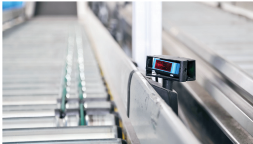
Both short-range CMOS, and this long-range, time-of-flight Wenglor photoelectric laser sensor, are often used in material handling applications.
