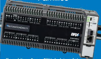
The revolutionary Do-more DM1 technology was first introduced in the H2 CPU as a next-generation CPU option for the longstanding DL205 PLC line. The newest addition, the BRX PLC, is the first platform designed specifically, from the ground up, for the Do-more engine.
