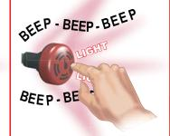
The audible signal can be silenced quickly by lightly pressing on the front of the indicator.
