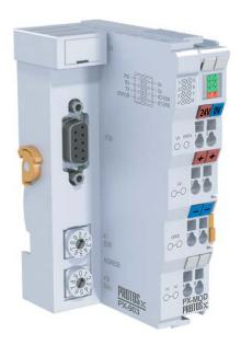
The PX-MOD Modbus RTU/ASCII Slave Bus Coupler allows connection of up to 64 terminals per assembly, 255 terminals total, in a Modbus RTU/ ASCII serial network. The PX-MOD communicates using high-level Modbus commands and supports 512 bytes of input data and 512 bytes of output data.
