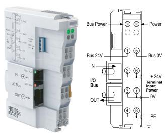
The PX-903 (type 4) Bus Expansion Coupler Terminal enables expansion of terminal assemblies. The PX-903 is installed at the beginning of an expansion terminal assembly and connects to a PX-902 Bus Expansion End Terminal or other PX-903 terminals.
