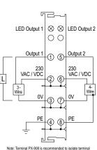
(WxHxD) (0.47 x 3.94 x 2.71 in) Adjacent Mounting on Bus Yes, 230 VAC/VDC only Terminals with Power Contact Adjacent Mounting on Bus No Terminals without Power Contact Passes Terminal Yes **Bus Power** Passes PE Bus Yes Agency UL/cUL File No. E157382, CE Approvals\* \*To obtain the most current agency approval information,
