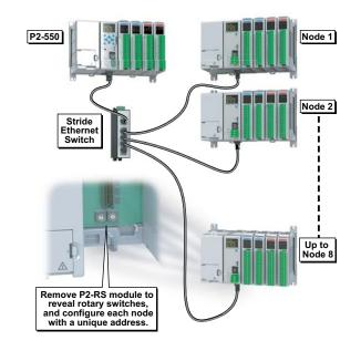
Add up to 8 Remote Bases using P2-RS Slave modules and up to 16 GS Drives on the Remote I/O Ethernet Network
