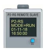
For user-defined messages, the display is configured using the Productivity Suite Programming Software. An LCD Page instruction allows the user to program text into user-defined tags and display the messages based on the ladder execution.
