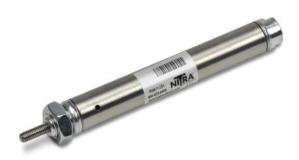
NITRA pneumatic stainless steel round body, interchangeable, non-repairable cylinder, 9/16 inch bore, #10-32 port, single acting, spring return, front nose mount.
