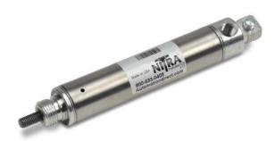
NITRA pneumatic stainless steel round body, interchangeable, non-repairable cylinder, 7/8 inch bore, 1/8 NPT port, single acting, spring return, rear pivot mount (pivot pin included).
