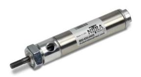
NITRA pneumatic stainless steel round body, interchangeable, non-repairable cylinder, 7/8 inch bore, 1/8 NPT ports, double acting, front nose mount
