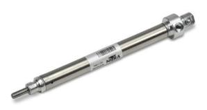
NITRA pneumatic stainless steel round body, interchangeable, non-repairable cylinder, 7/16 inch bore, #10-32 port, single acting, spring return, rear pivot mount (pivot pin included).
