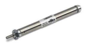
NITRA pneumatic stainless steel round body, interchangeable, non-repairable cylinder, 7/16 inch bore, #10-32 port, single acting, spring return, front nose mount.
