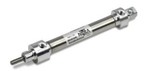
NITRA pneumatic stainless steel round body, interchangeable, non-repairable cylinder, 7/16 inch bore, #10-32 ports, double acting, rear pivot mount (pivot pin included).
